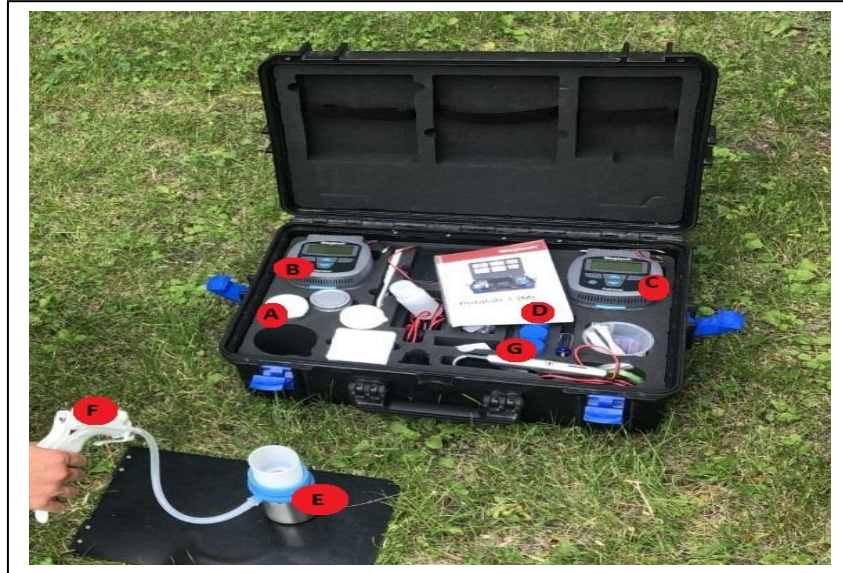
Figure 4: Palintest Potalab®+ (M) Advanced Portable Water Quality Laboratory. Included are: A- Absorbent Pads; B & C- Petri Dishes (in incubator); D- Instruction Manual; E- Membrane Filtration Unit; F- Hand Vacuum Pump; and G- Media Measuring Device (MMD).
